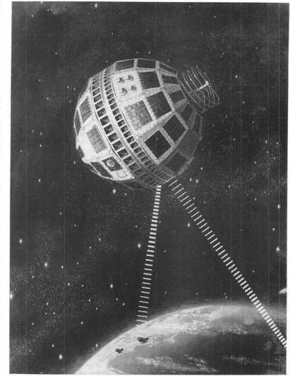
IN ORBIT AND ACTION — An artist's version shows Telstar transmitting messages over the Atlantic Ocean. Power for Telstar comes from 19 nickel-cadmium cells charged by solar cells which convert sun's energy.
